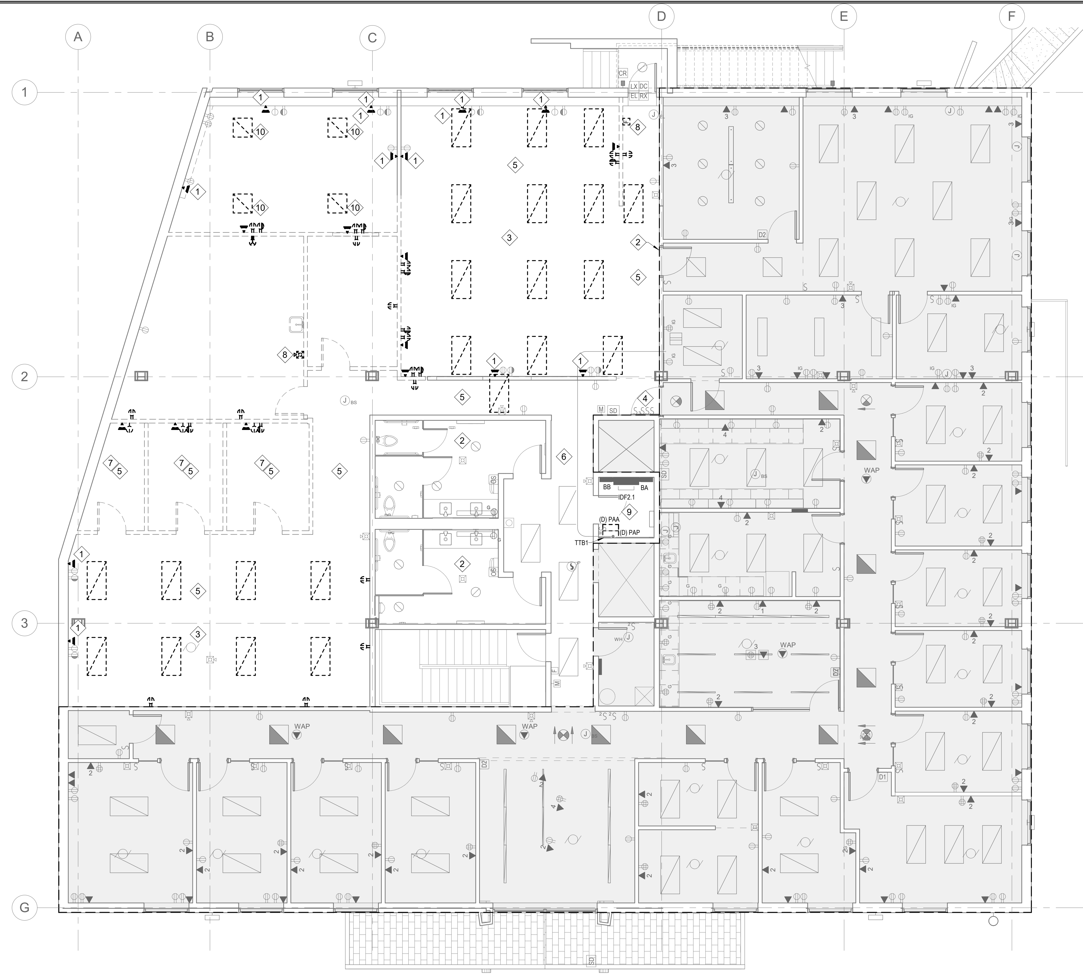
1 SECOND FLOOR DEMOLITION PLAN E112 SCALE: 3/16" = 1'-0"
